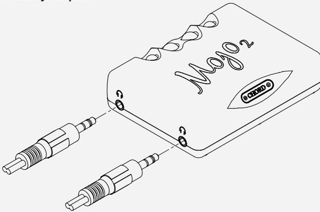
Connect up to two pairs of (3.5 mm mini-jack) headphones to Mojo 2, simultaneously. The device's volume control (see section 6.8) will adjust both headphone outputs together (there is no independent volume control for each headphone).
