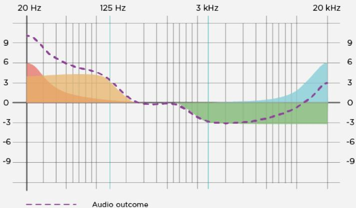
Graph 3 overlays common musical instruments on the frequency spectrum, in a very broad sense, demonstrating how the prominence of instruments might be affected when making adjustments using the DSP tone controls. It is not definitive and is a guide for experimentation only.
